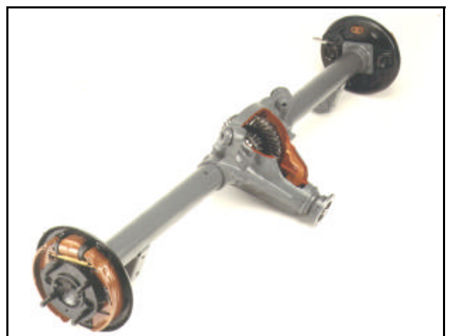
SECTIONED REAR AXLE (P2231)
