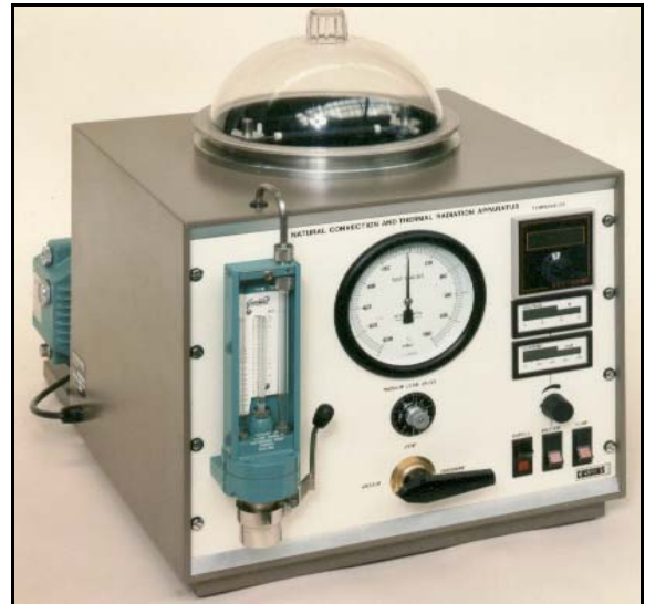
P3300 allows the convection heat transfer to be reduced by reducing the air pressure, whilst radiated heat is still transferred
