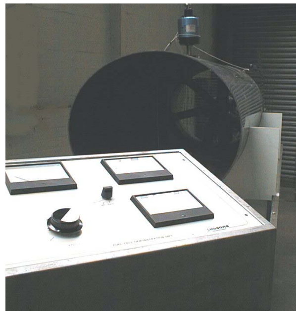
P3105 & 6 Wind channel & bench with VAWT
